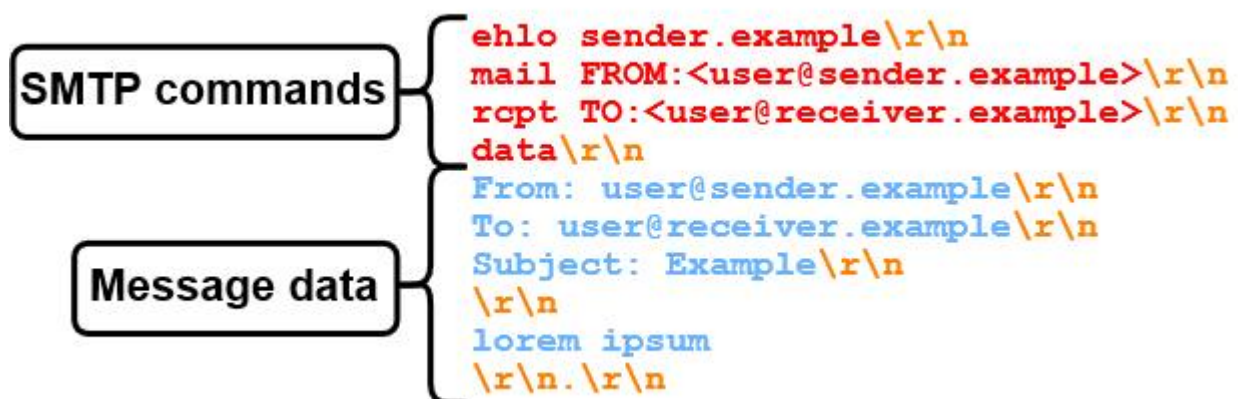
• Figure 7: SMTP session with SMTP commands and message data separated by colour. *
